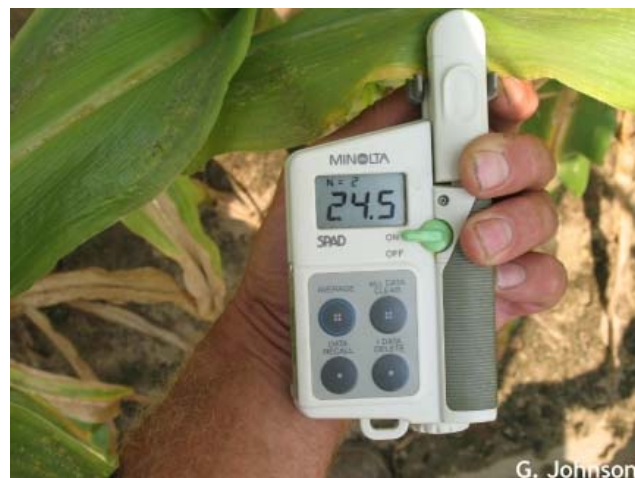
Chlorophyll meter reading on the ear leaf of a N deficient plant. The reading on this plant was more than 50% lower than plants without N deficiency symptoms in an adjacent field.
